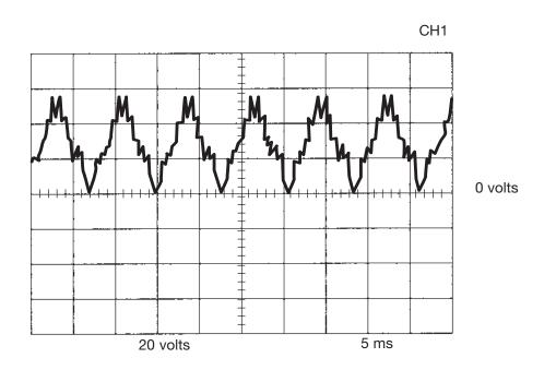
This is the typical CV output voltage generated from a properly operating machine. Note that each vertical division represents 20 volts and that each horizontal division represents 5 milliseconds in time.
